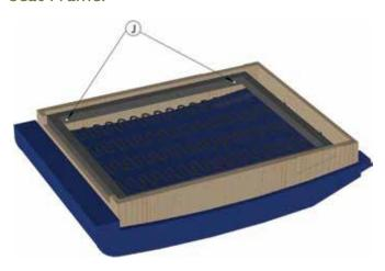
**J**: Using the Robertson screwdriver, remove the 4 wood screws which attach the seat frame to the seat cushion frame.
