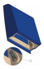
**I:** Using the Philips screwdriver, remove the machine screws securing metal KD brackets.
