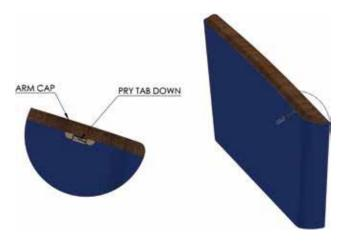
K: If the chair has arm caps, toward the outside rear of the arm cap is a small gap between the arm cap and the upholstered side. You will need to feel for it. Using the flat blade screwdriver, as shown above, locate and pry down the metal clip securing the arm cap pin. Using the hammer, you should then be able to knock the arm cap forward and out of the clips. If you are not able to remove the arm caps, you will need to break them away from the end frames.
