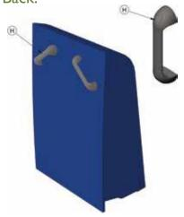
H: Using a knife, pop the small caps on the back of the push handles. Remove the cap screws with a 3/16" Allen key.
