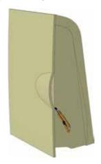
For all of the upholstered components, the fastest way to remove the fabric is to run a knife next to every staple line, rather than pull every staple, as this would take much longer! The fabric can then be peeled our pulled back.
