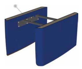
**D:** With the Philips screwdriver, remove the pan head 8 machine screws that secure each end frames. Lay the end frames to one side.
