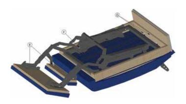
**E & F:** Using the Philips screwdriver, the next step is to remove the 8 machine screws that secure the leg rest and the intermediate flipper. Next remove the 4 machine screws securing the seat frame, and lay the seat frame to one side.
