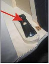
A: As shown in the left photo above, raise the rear flap and lift the latches (right photo) that secure the recliner back. The easiest way is to release the catch on one side, have your assistant lift that side up slightly, and then repeat on the other side. The back will then lift straight up. Lay the back to one side.
