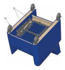
B: With an assistant, tip the recliner over on its front. If equipped with casters, use the ¼" Allen key to remove the four casters. If equipped with wood legs, remove the nylon glides from the bottom of each leg, and then unscrew the legs. Use the Channel lock pliers to loosen them, if needed. If available, secure the hanger bolts of each leg in a bench vise, and unscrew the hanger bolt from the leg.
